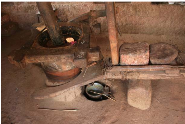
Traditional wooden machine of oil extraction
