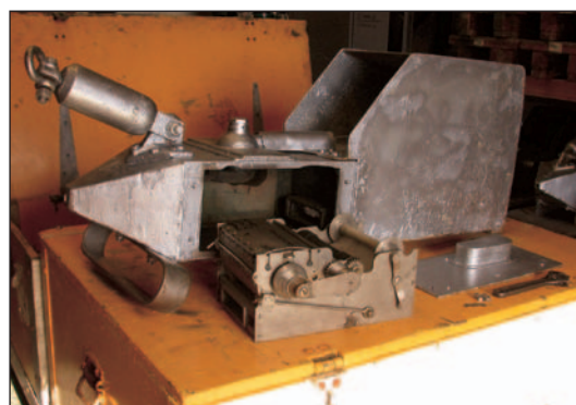
Figure 2.1. Photograph of a Continuous Plankton Recorder with the sampling cassette removed to show the silk spool and preservative storage tank. The cassette has been reversed to show the ingenious fusee tension mechanism on the side that takes up slack in the silk as it is wound on
