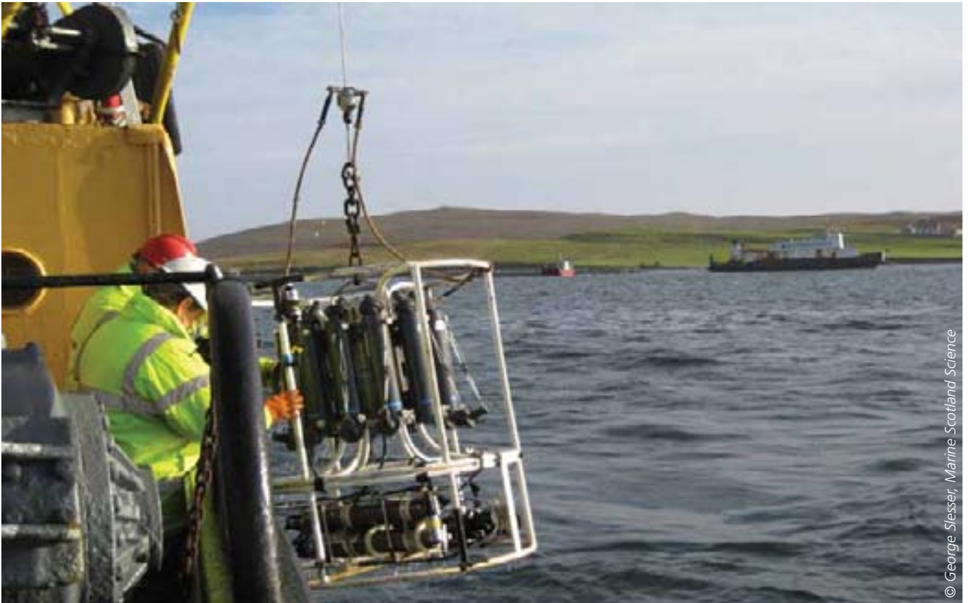
Equipment used to collect water samples and measure a range of variables including temperature
