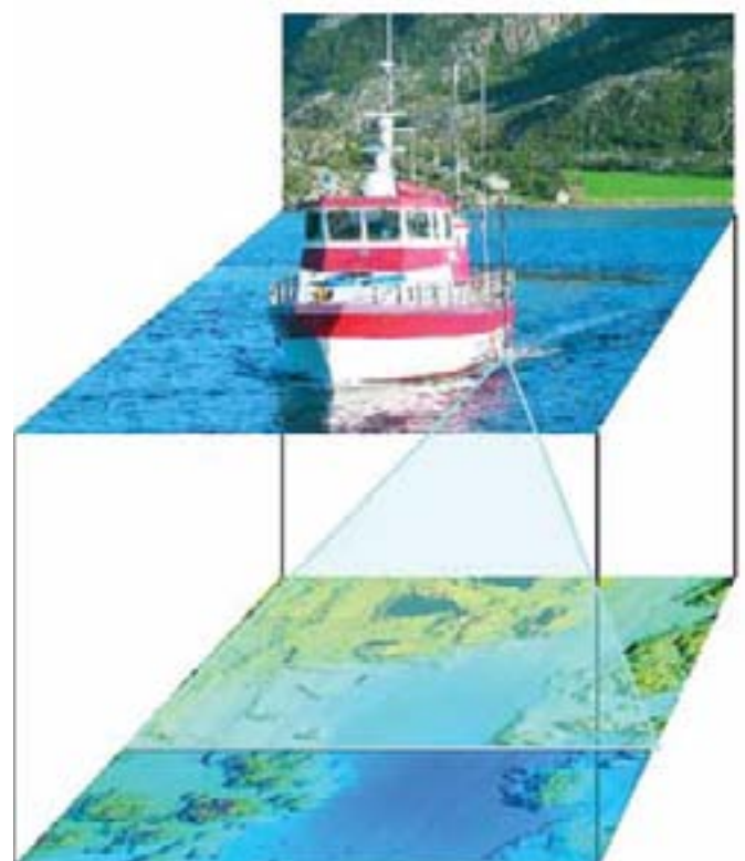
Figure 2.5 Schematic illustration demonstrating the principles of data collection using Multibeam Echosounder Systems.
